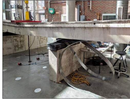
Figure 4-25: Load-displacement response and image of SCS4 at failure
