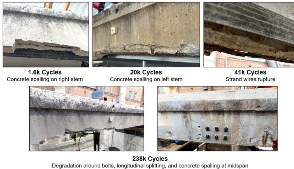
Figure 4-21: Images of WCS3 at various stages of loading
