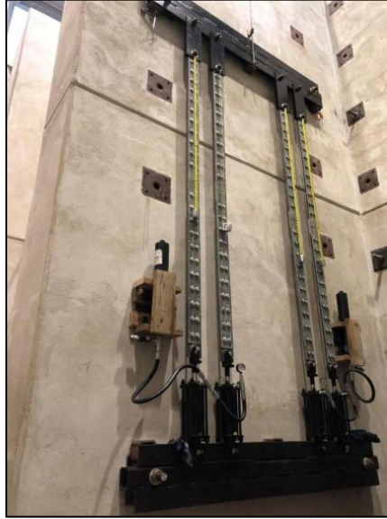
Figure 2-2: Sustained loading test setup (adapted from (Bourara, 2019)).
