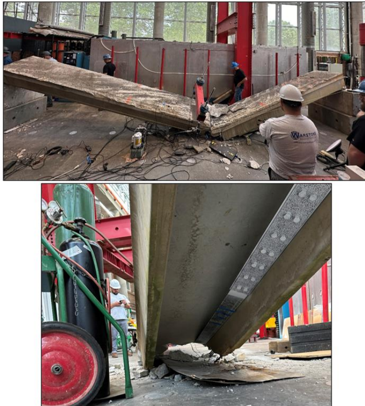
Figure 4-8: Images of WCS1 at failure
