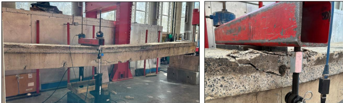
Figure 4-3: Specimen SCU2 at failure
