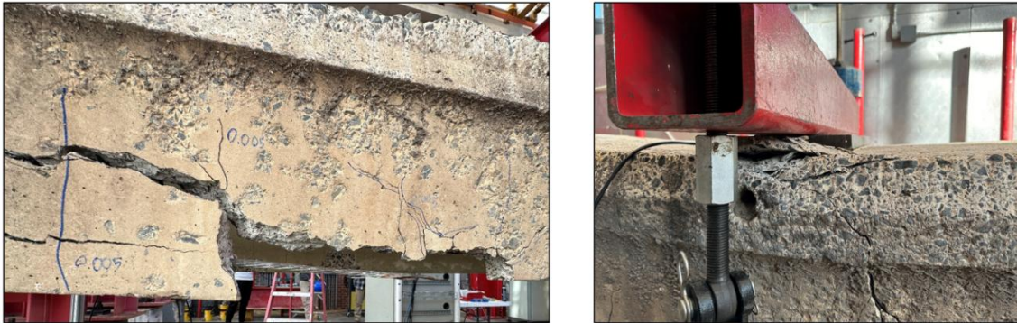
Figure 4-2: Specimen SCU1 at failure
